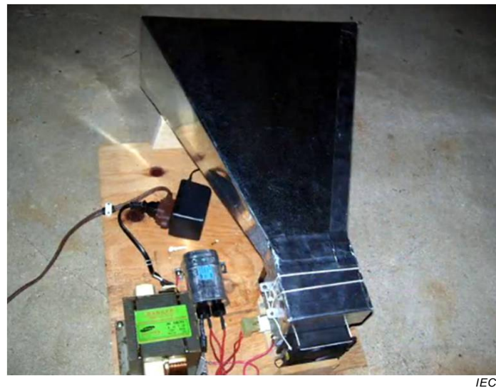
Figure B.9 – A do-it-yourself electromagnetic weapon made from an oven magnetron [13]
